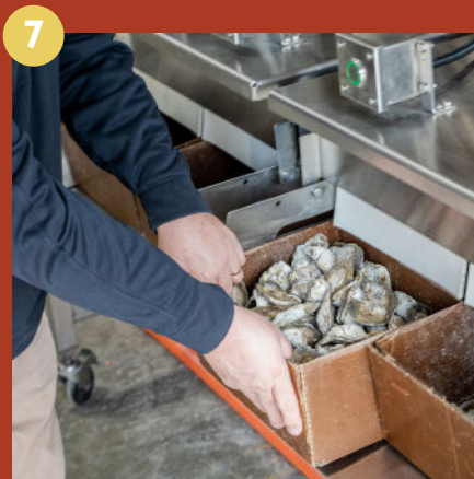
7 OysterLogic program tracks graded oysters and stops system with alarm if no boxes are available allowing operator to replace and restart system with no product loss.
