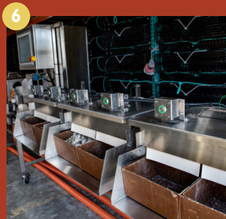
6 Integrated sensors confirm and guarantee oyster count; stations flash green once predetermined number of oysters are counted.
