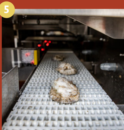
5 Six air nozzles move oysters quickly and gently to one of six pre-set stations for boxing or bagging.
