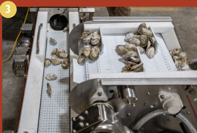
3 Cross-feed delivers oysters to the singulator tube where they are turned on two points and accelerated onto the conveyor for precise laser grading.
