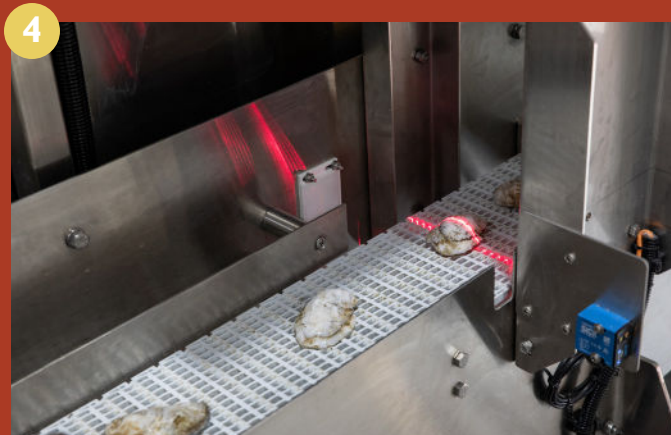
4 After emerging from the singulator, oysters are graded and sorted by highly accurate laser sensors.
