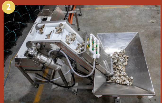
Vibrating, self-loading up-feed features quickly moves oysters up a conveying elevator with staggered flights for steady loading.
