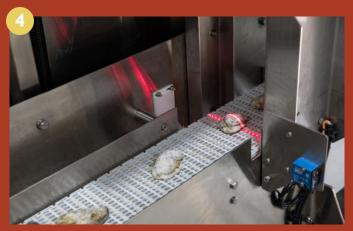
After emerging from the singulator, oysters are graded and sorted by highly accurate laser sensors.
