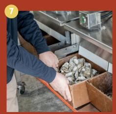
OysterLogic program tracks graded oysters and stops system with alarm if no boxes are available allowing operator to replace and restart system with no product loss.
