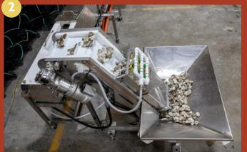
Vibrating, self-loading up-feed features quickly moves oysters up a conveying elevator with staggered flights for steady loading.
