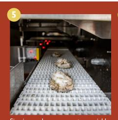
Six air nozzles move oysters quickly and gently to one of six pre-set stations for boxing or bagging.
