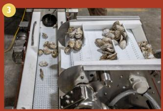
Cross-feed delivers oysters to the singulator tube where they are turned on two points and accelerated onto the conveyor for precise laser grading.
