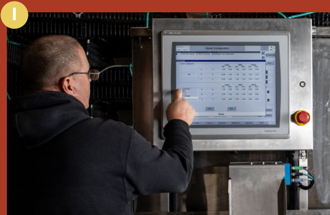
Large touch-screen monitor and intuitive interface features seven distinct screens to configure, operate and manage processing for different levels of authority.
